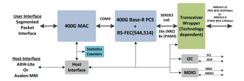
The 400Gbps Ethernet IP solution offers a fully integrated IEEE802.3bs compliant solution for use in core networks, Ethernet switching and network interface card (NIC) applications. The Ethernet cores implement an efficient architecture to achieve best in class resource utilization and performance numbers for targeting the complete 400Gbps Ethernet solution to ASICs as well as FPGAs.
