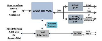
A complete reference design using a simple L2 (MAC level) packet generator/checker is also included to facilitate quick integration of the Ethernet MAC in a user design.
