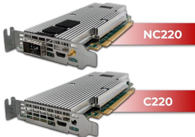
High performance Data Center accelerator and edge AI low profile PCIe card with Intel's 10nm Agilex FPGA
