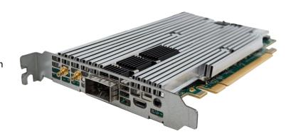
High performance Data Center accelerator, edge AI and 5G DU/CU low profile PCIe card with Intel's 10nm Agilex FPGA.
